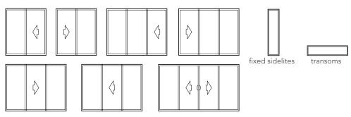
Only available in 2-panel configuration in Certified Wind Load areas. Sidelites and transoms must be installed in a separate opening or use approved engineering mulls.
