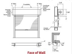
Maintains clearance of full opening, minimal exposed components
