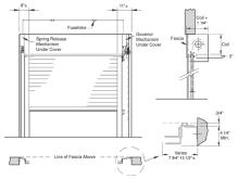
**Between Jambs** Mounts within the opening, fascia (front hood closure piece) required.
